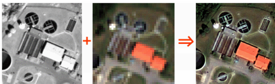
Figure 1.1: Image pan-sharpening with QuickBird images. The left and middle input images are obtained from DigitalGlobe, and the right-hand image is the fused result from HighView . All images are subject to the same histogram stretch.
